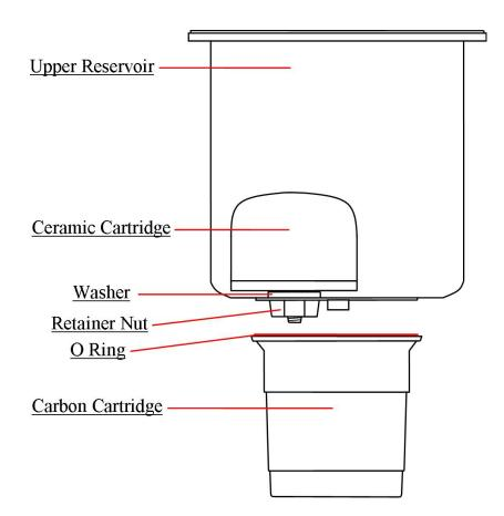
The Ceramic Cartridge is fragile. Handle it with care. • Prime the Cartridge by soaking it in water for 2 hours or overnight.
