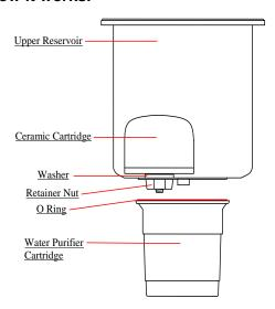
The upper reservoir is filled with tap water. The water is first filtered by the Ceramic Cartridge and then by the Water Purifier Cartridge as it flows through to the lower reservoir.
