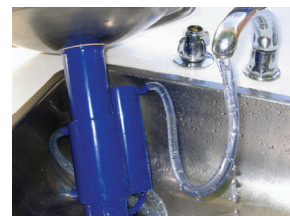
Flush condenser via tube
